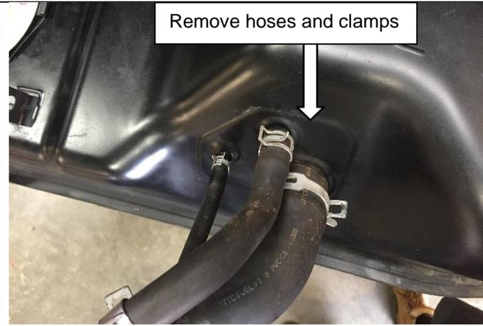
Remove fill hoses from the original fuel tank, retain the hoses and clamps for the installation procedure.
