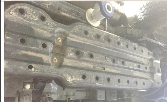
Remove 4 x M8 nuts retaining plastic stone shield and remove shield.
