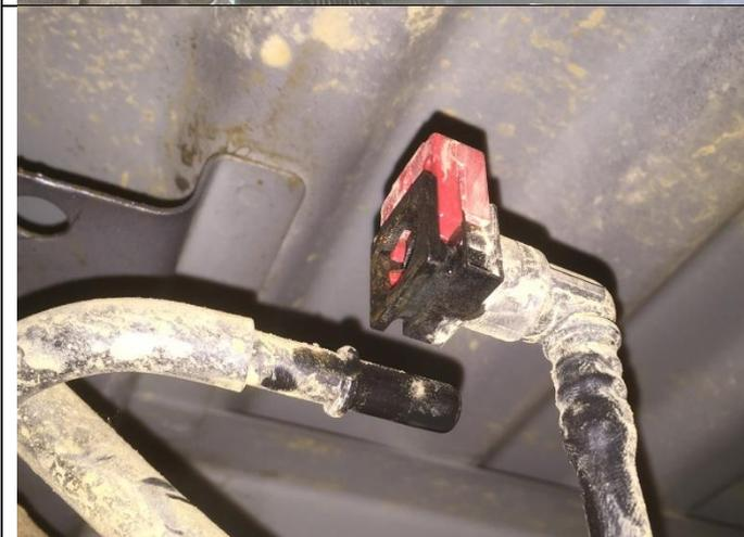
Disconnect the fuel return line on the fuel cooler or chassis if no cooler fitted at the rear of the fuel tank.
