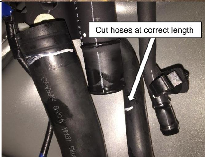
Mark and cut the 35mm and 16mm fuel hoses to line up with the filler neck.
