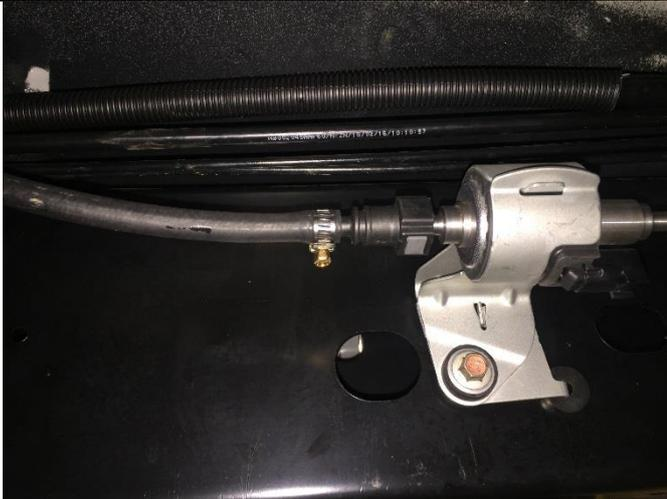
Install a straight female quick connect fitting to the other end of the 1100mm fuel hose supplied in kit and secure with a hose clamp.
