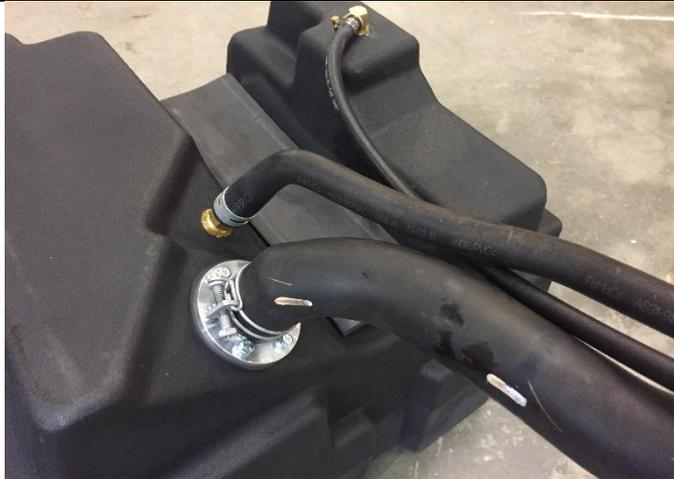
Install the 35mm and 16mm hoses onto the new tank and secure with clamps retained during removal.
