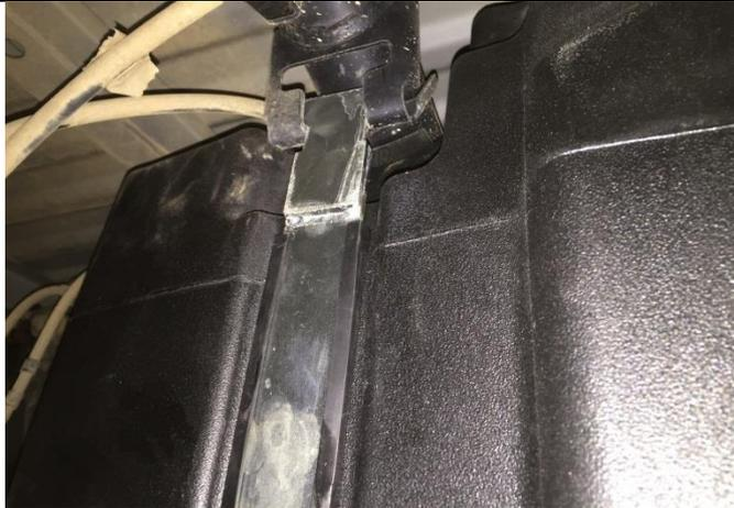
Insert the hook end of the rear mount strap into the saddle in the chassis. Swing the strap around the tank and secure using the bolts retained from the removal procedure.
