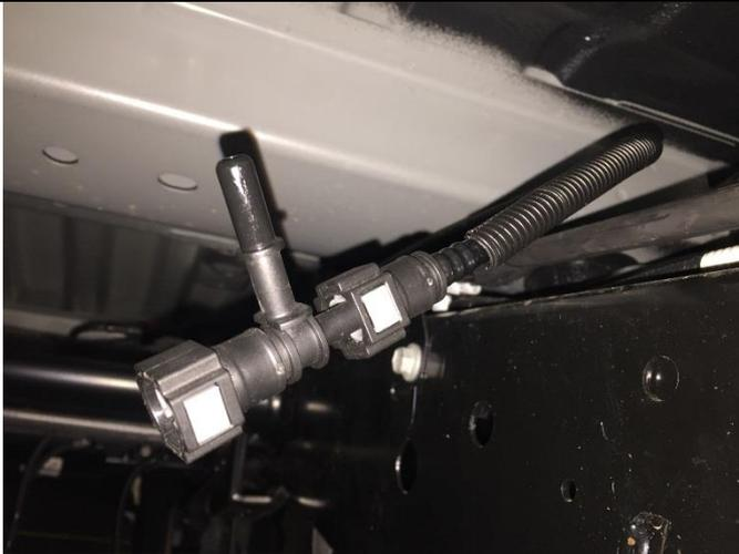
If the vehicle being installed has a Diesel Particulate Filter (DPF) fitted that incorporates an auxiliary fuel pump mounted on the LH chassis rail, it will be necessary to install the T piece adaptor to the return line at the tank end.
