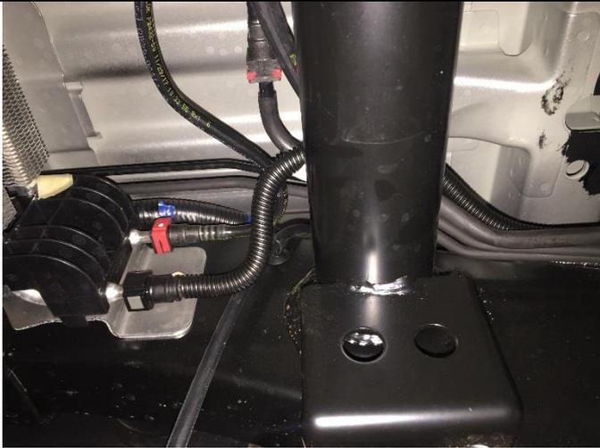
Install the 2 pieces of split tubing supplied in the kit over the top of the new fuel lines supplied in the kit prior to installing fuel lines into vehicle.
