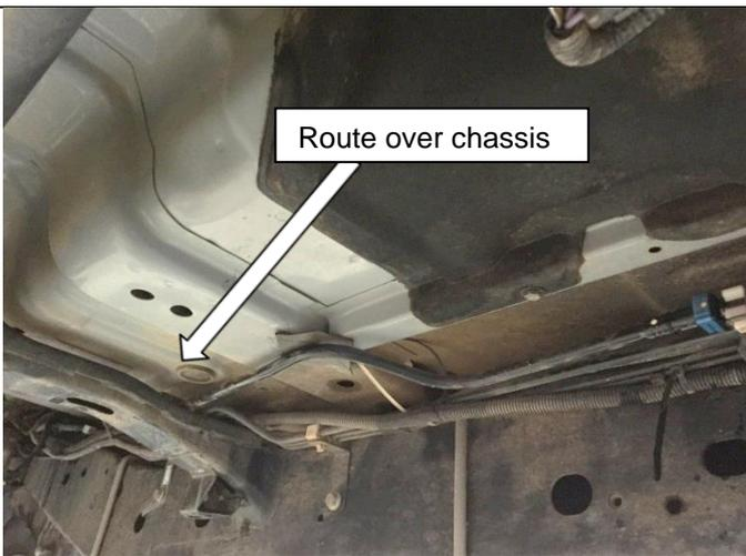
Connect the new 12mm diameter fuel line to the original fuel line located on the LH chassis in front of the tank.
