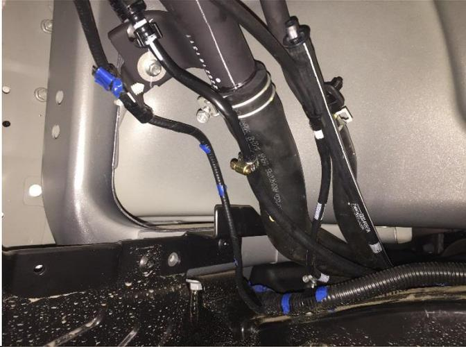
Reconnect the 35mm and 16mm hoses to the fuel filler neck. Secure using original clamps retained from the removal procedure.
