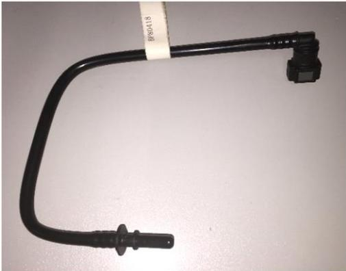
If the vehicle being fitted does not have a fuel cooler, use the horseshoe shaped fuel line supplied in the kit.
