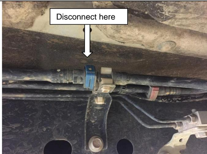
Disconnect the fuel supply line ( blue clip ) at the point shown in front of the fuel tank on the LH chassis rail.
