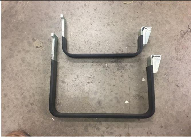
Install the 40mm wide rubber extrusion included in the kit onto the mounting straps as shown. Ensure that the rubber is covering the straps evenly and that all radii are covered.
