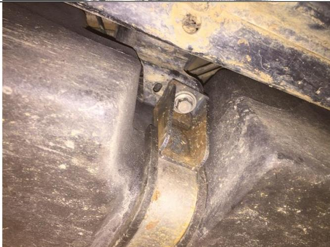
Insert the hook end of the front mount strap into the saddle in the chassis. Swing the strap around the tank and secure using the bolts retained from the removal procedure.
