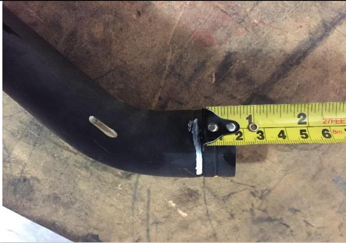
Cut 20mm from the tank end of the 35mm fill hose.
