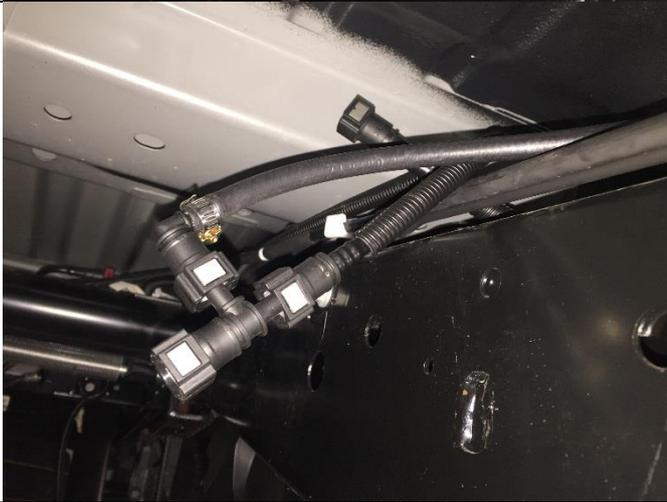
Assemble 1 x 90 degree female quick connect fitting into the 1100mm length of hose and secure with a clamp supplied in the kit.
