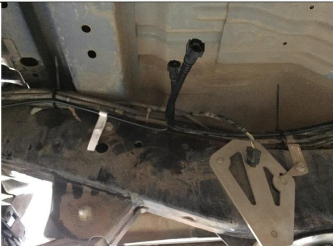
The 2 fuel pump ends of the supply and return lines should now be positioned next to each other.
