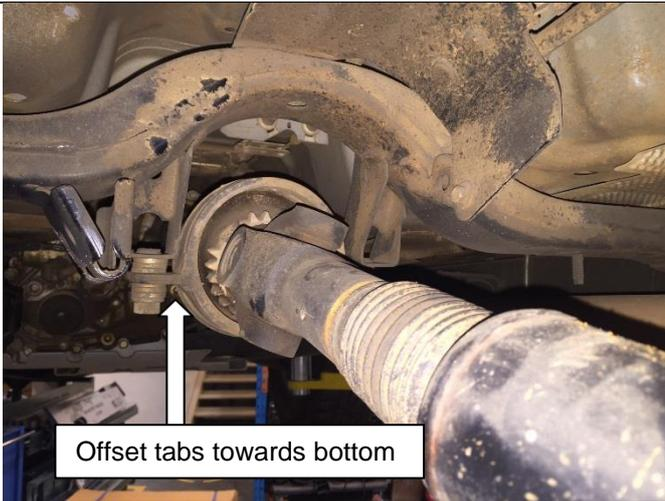
At this stage ensure correct orientation of the tailshaft centre bearing. The mounting tabs are offset and are to be positioned as shown.
