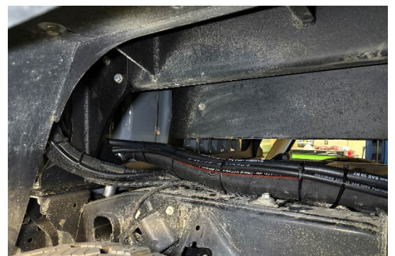
Photo 12: Connect the filler hose
