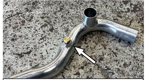
Photo 9: Install Brass Plug
