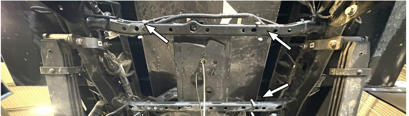
Photo 13: Prep Auxiliary tank area
