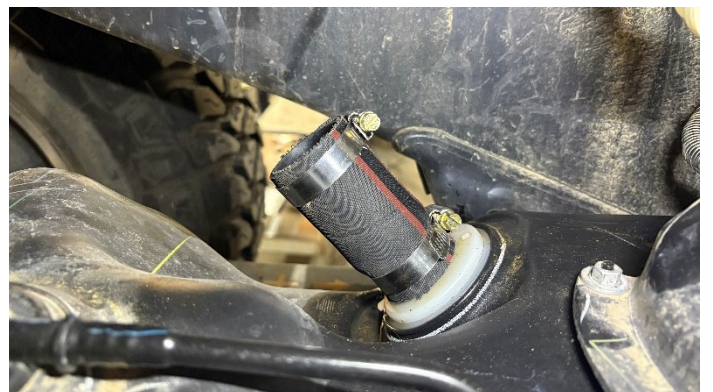
Photo 8: Install Filler Hose
